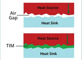
TIMs have high thermal conductivity and are compressible, filling in air gaps to improve heat transfer from the heat source to the heat sink component.
