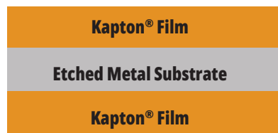
All Polyimide Adhesiveless (Fralock's Adhesiveless Lamination Technology ALT™)
